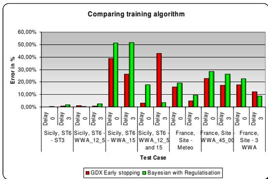
It can be seen clearly that in the Sicilian case obviously using ST6 as long term data leads to extremely good results – as well as the first World Wind Atlas grid point. The second one, located 15° east leads to bad results and obviously is not a good choice for long term correlation at all.
