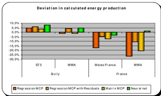
It can be seen, that for the Sicilian case no significant change in the result quality occurs – all methods deliver good results. The French case shows clear improvements by using the neural network, especially when using the World Wind Atlas data.
