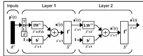
Structure of a two layer focussed time delay neural network.
